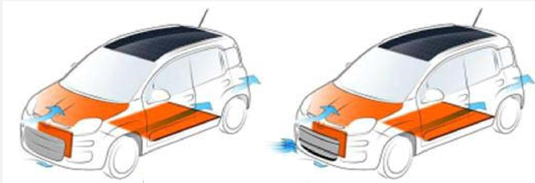
A redesign of the front part of the car is needed, by the substitution of the front radiator or with higher efficiency systems
