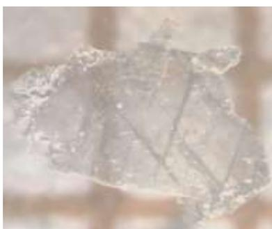
**Figure 1:** Optical image of a few millimeters side hBN crystal
