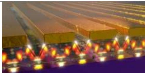
**Figure 1:** Schematic of the 2D polaritonic nanoresonator that show the field intensity of the propagating mode.
