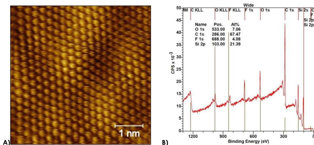
**Figure 1:** A: Atomic resolution preliminary unfiltered STM image of fluorinated graphene showing preserved graphene-like structure. B: Wide XPS spectrum of the fluorinated sample, showing the presence of fluorine and proportion of fluorine and carbon.
