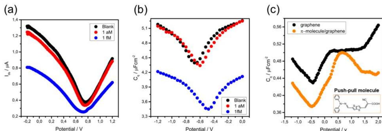
**Figure 1:** (a) Transfer curves obtained in DC transistor mode, (b) quantum capacitance response in functions of the electric potential resolved in AC electrochemical mode for two concentrations of target-DNA in PBS. (c) The electronic structure effect of the push-pull  $\pi$ -conjugated molecule appears as a modulation of graphene quantum capacitance trace.
