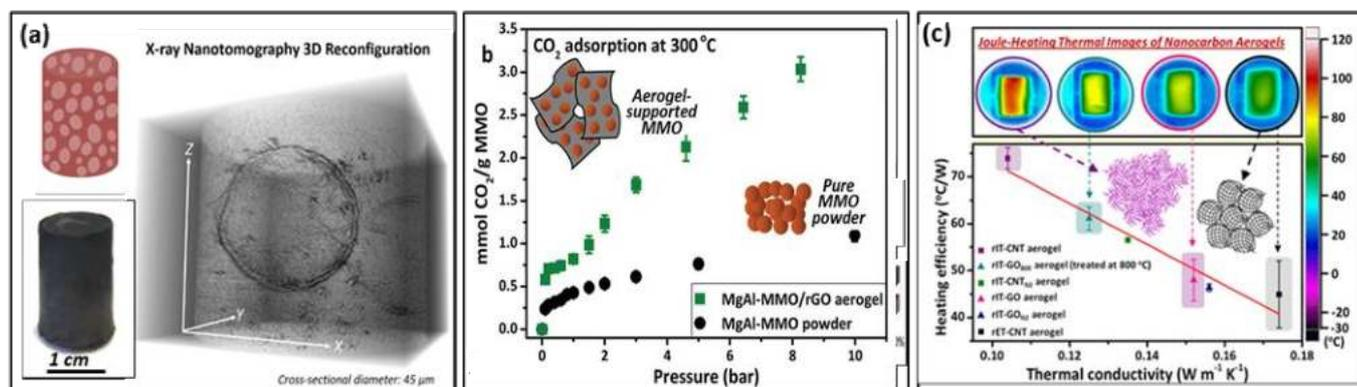
**Figure 1:** (a) X-ray nanotomography of an emulsion-templated nanocarbon aerogel catalyst; (b) High-pressure CO<sub>2</sub> capture performance of rGO aerogels functionalised with mixed-metal-oxide (MMO) nanoparticles; (c) Thermo-electric structure-property relationship study of different nanocarbon aerogels.
