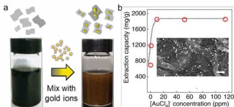
**Figure 1:** Gold extraction by rGO. (a) Schematic of the extraction process using rGO. After mixed with gold ion, rGO suspension gradually changed its color from black to brown. (b) Extraction capacity as a function of gold concentration after 24 h. Inset is a Scanning electron microscopy image of reduced gold nanoparticles adsorbed on rGO. Scale bar is 500 nm.
