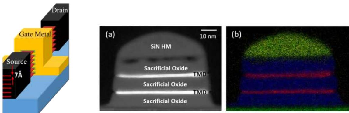
**Figure 1:** Schematic of Ultimate CMOS scaling with stacked 2D nano-sheets, followed by (a) TEM cross section of a two-layer TMD stacked nanoribbon structure showing 2 – 3 ML per nanoribbon, (b) TEM elemental mapping of stacked 2D nanoribbons.
