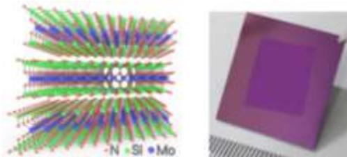
**Figure 1:** The structure of MoSi<sub>2</sub>N<sub>4</sub> and a monolayer MoSi<sub>2</sub>N<sub>4</sub> film grown by chemical vapor deposition.
