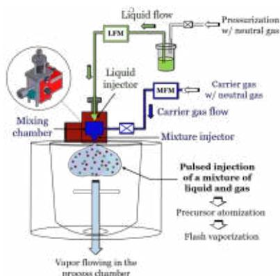
**Figure 1:** Schematic representation of KEMSTREAM's two-stage DLI system
