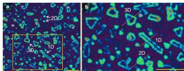
**Figure 1:** (a) SHG map of the MoS<sub>2</sub> nanostructures and (b) zoom over a selected area with edge-enhanced SHG.
