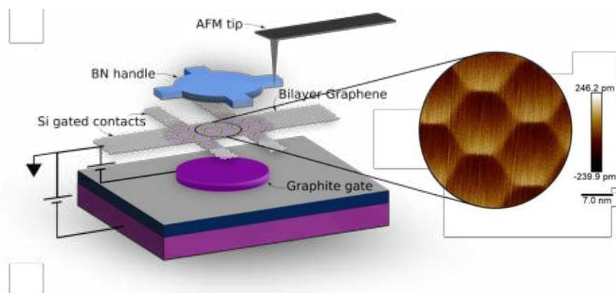
**Figure:** Schematics of our rotatable van der Waals heterostructure and AFM image of a bilayer graphene/BN moiré superlattice.
