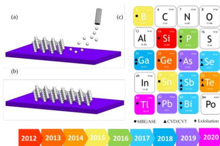
**Figure 1:** (a)-(b) sketches of the Xene synthesis on a substrate. (c) The periodic table of Xene discovered so far (from 2012 to 2020) and the methods (MBE-CVD-Exfoliation) used for their synthesis. Figure adapted from [1].
