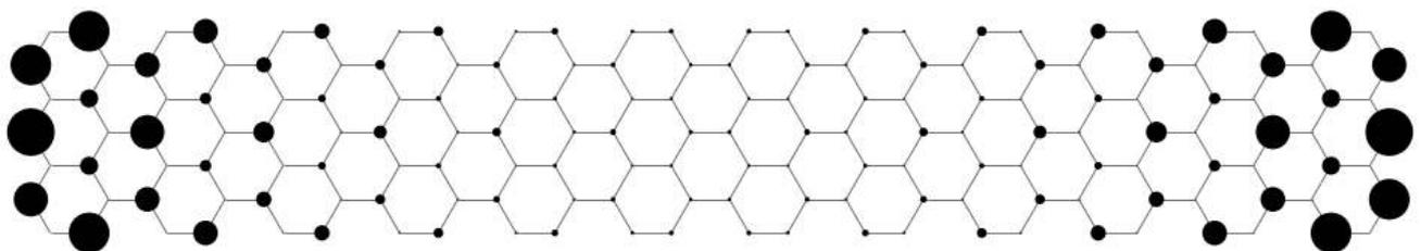
**Figure 1:** Electronic density of a topological end-states in a 7-atom width armchair graphene nanoribbon. The size of the dots is proportional to the mean densities of electrons.
