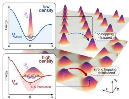
**Figure 1:** The moiré potential captures excitons within its minima creating arrays of localized excitons. For large densities the inter-excitonic repulsion gives rise to a decreased effective potential and a change of the exciton wave function with far-reaching consequences for optical properties and exciton transport.
