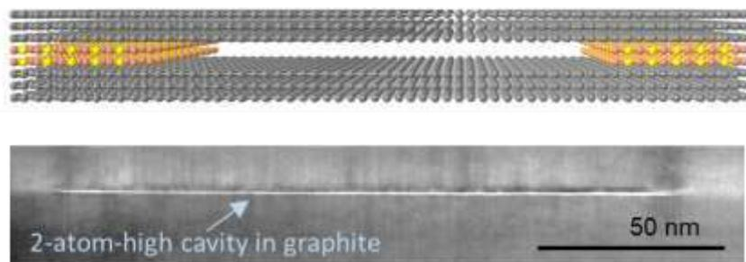
**Figure 1:** (Top) Artist's impression: Angstrom-scale cavities with atomically flat walls can be made from different materials and have different heights. (Bottom) Transmission electron micrograph of a 2D cavity in graphite with a nominal height of 6.7 Å. It is made by placing strips of bilayer graphene between two atomically-flat graphite crystals.
