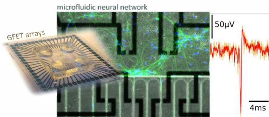
**Figure 1:** Neuron-gated GFET arrays with microfluidic circuits (left) allows for highly efficient extra-cellular detection of action potential (right). The graphene sensing site being optically transparent, cells can be observed in real-time during the culture (several weeks) providing multiple way to follow both structural and functional changes within model neural network (center).
