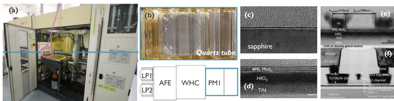
**Figure 1:** (a) tool mainframe, (b) cross-flow reactor and layout, growth on (c) either sapphire aiming a subsequent transfer to the final substrate or (d) directly on amorphous dielectric, either the gate dielectric or a sacrificial material to pursue the integration on same substrate. Cross section of lab (e) and fab (f) devices.
