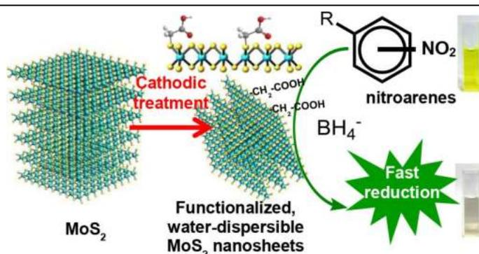
**Figure 1:** Scheme of the electrochemical cathodic strategy used to obtain derivatized 2H-MoS<sub>2</sub> dispersions and its application to the reduction reaction of several nitroarenes and organic dyes.
