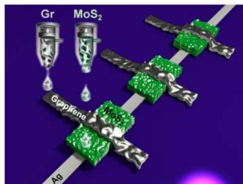
Schematic of fully printed Ag/MoS<sub>2</sub>/Gr memristors.
