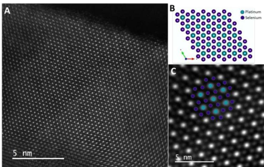
**Figure 1:** (a) Atomic resolution HAADF image of LPE PtSe<sub>2</sub> (b) Model of PtSe<sub>2</sub> preferential 1T structure (c) Z-contrast showing clear 1T structure of PtSe<sub>2</sub>.
