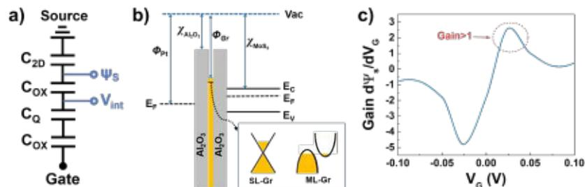
**Figure 2:** (a) Capacitor divider model and (b) band diagram of the gate stack. (c) Simulation results.
