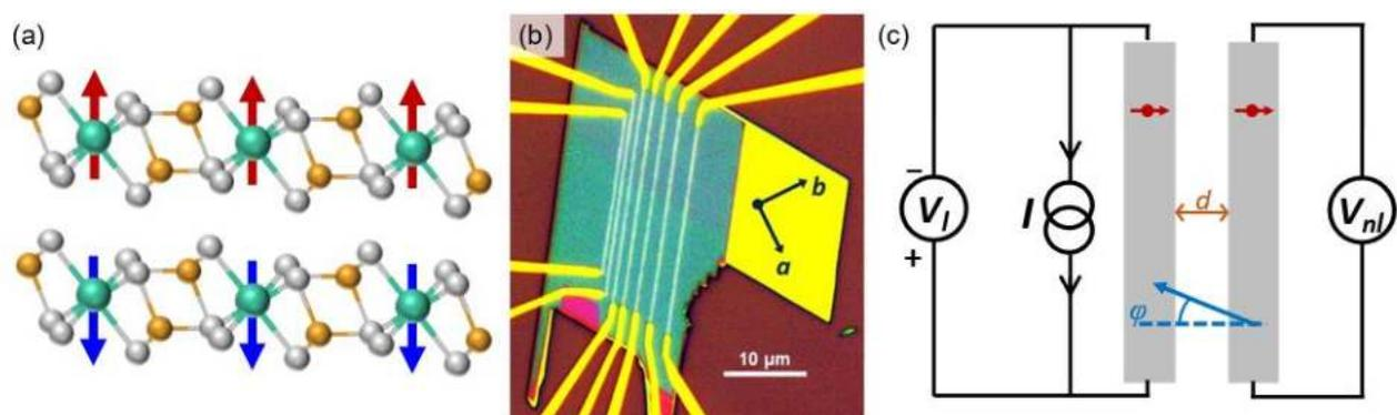
**Figure 1:** a) Bilayer of CrPS<sub>4</sub>, arrows representing magnetic moments, b) optical image of device with Pt contacts on CrPS<sub>4</sub> flake, c) Circuitry of non-local measurements.
