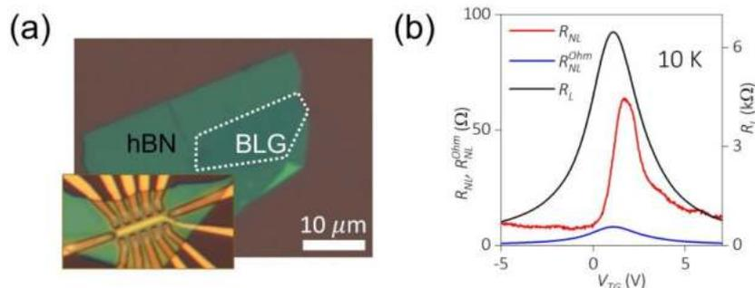
**Figure 1:** (a) hBN/bilayer graphene heterostructure with the edges aligned. Inset: Optical image of the final device. (b) Measured local ( $R_L$ ) and non-local ( $R_{NL}$ ) resistance for the heterostructure.
