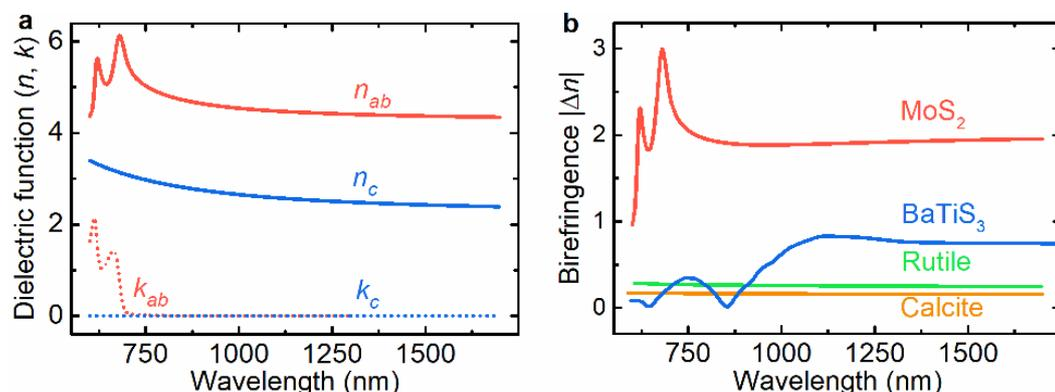
**Figure 1:** **a.** Optical constants of MoS<sub>2</sub>. **b.** Birefringence of MoS<sub>2</sub> in comparison with other anisotropic materials.
