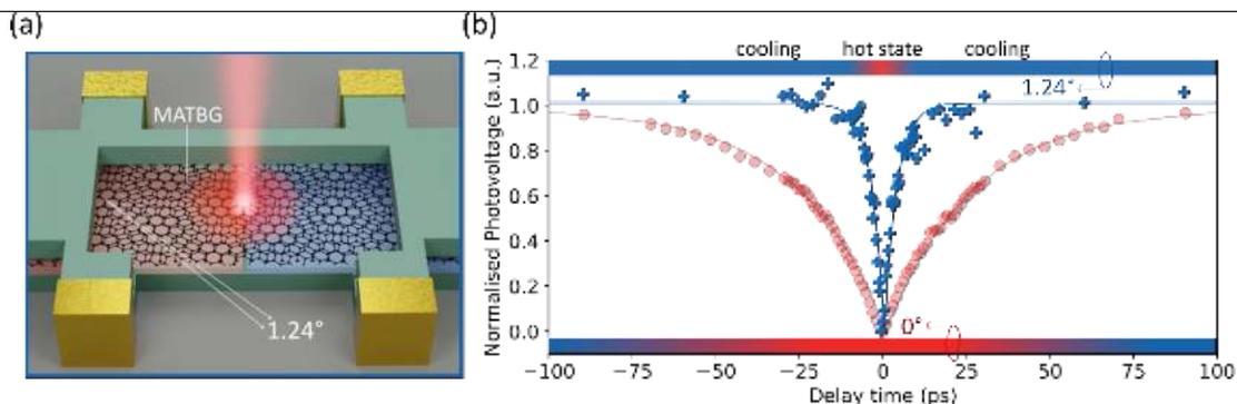
**Figure 1:** (a) Illustration of the hBN-encapsulated MATBG device. We generate a photovoltage by illuminating the pn-junction (red/blue regions). (b) Controlling the time delay between two ultrafast pulses reveals the hot carrier cooling dynamics. At low temperatures, these are significantly faster in the case of MATBG ( $1.24^\circ$ ) than non-twisted BLG ( $0^\circ$ ).
