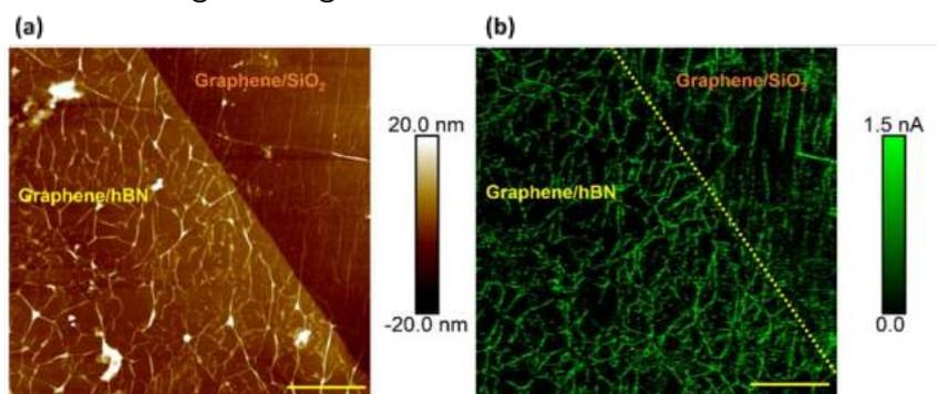
Figure: (a) Topography of CVD graphene transferred on top exfoliated 10-layer hBN through wet transfer. (b) Current mapping of CVD graphene on 10-layer hBN and SiO<sub>2</sub>/Si areas. Dashed yellow line denotes the edge of the graphene/hBN heterostructure. Scale bars are 2 μm.
