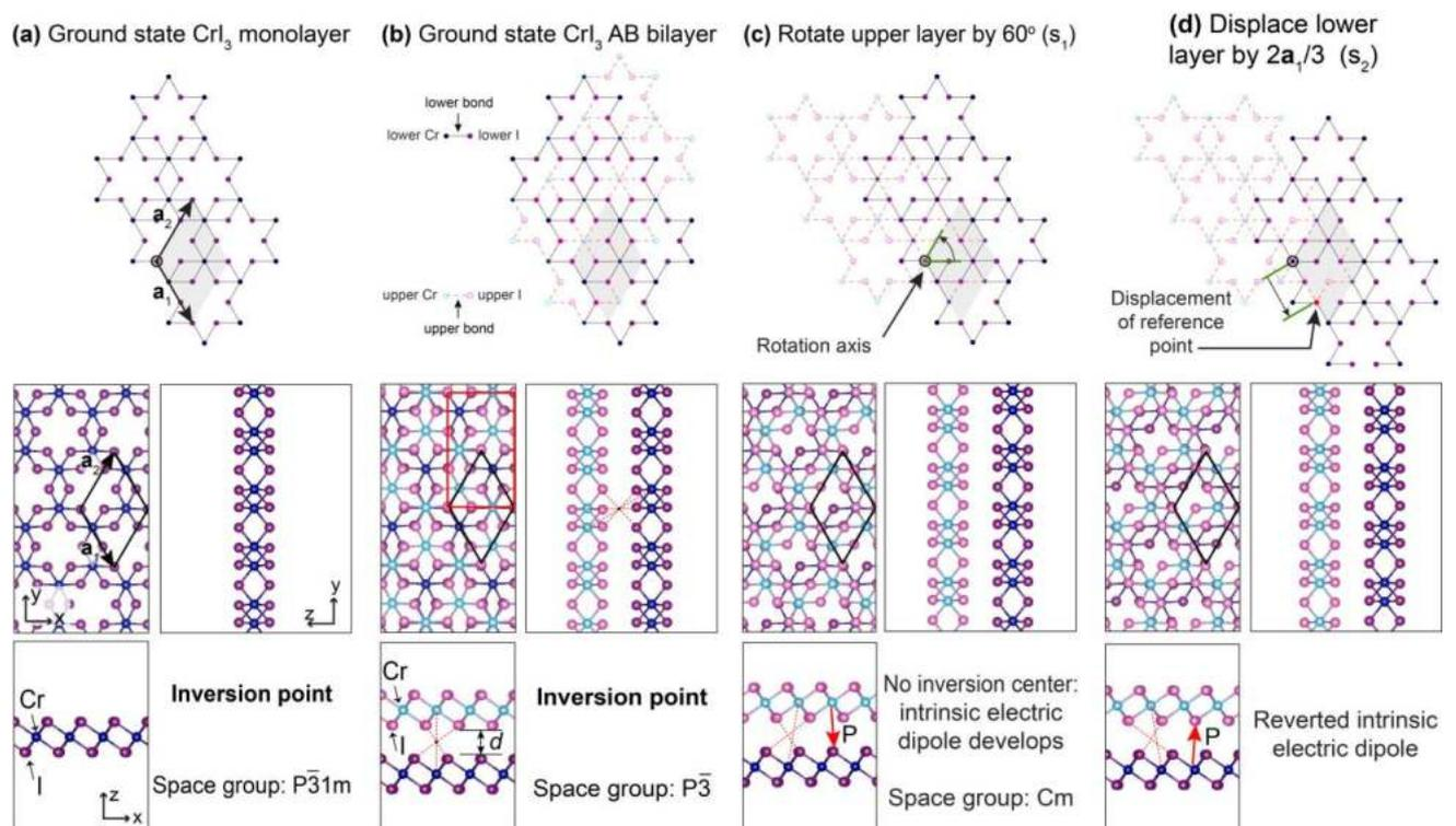
**Figure 1:** Process to enhance the magnetoelectric coupling on a CrI<sub>3</sub> bilayer.
