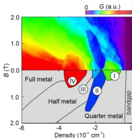
**Figure 1:** Conductance map as a function of charge carrier density and magnetic field B at a large electric displacement field measured in encapsulated bilayer graphene at a temperature of 10 mK. Several correlated phases of Stoner (quarter metal and half metal) and non-Stoner type (phases I-IV) appear.
