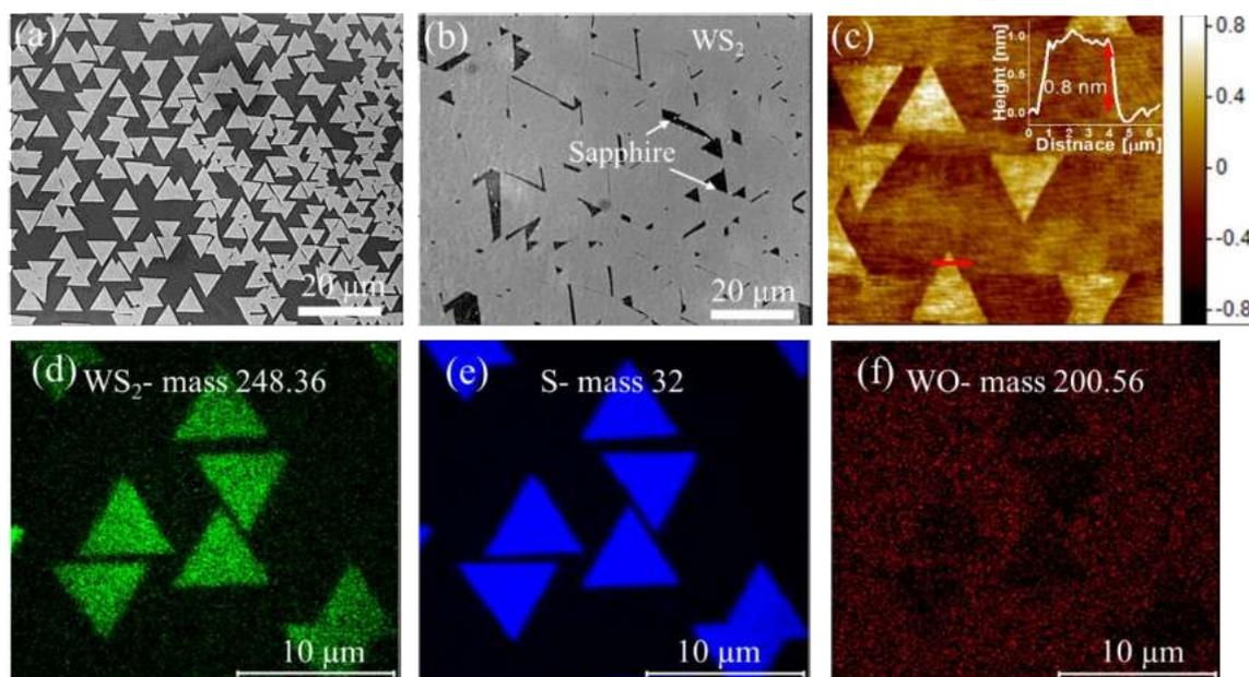
**Figure 1:** WS<sub>2</sub> epitaxial growth on sapphire (a-b) optical image; (c) AFM image; (d-f) TOF-SIMS analysis showing the domain and the WO<sub>x</sub> interface layer between WS<sub>2</sub> to the sapphire.
