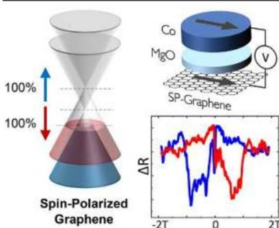
**Figure 1:** (Left) Exchange-induced spin splitting of the graphene Dirac cones by proximity effect. (Upper right) Device concept of magnetic tunnel junction with magnetized graphene as spin polarizer. (Lower right) Typical spin signal recorder on one of our devices
