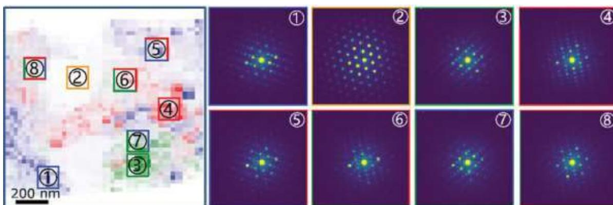
**Figure 1:** 4D STEM (scanning electron diffraction analysis of intercalation ordering in KMoS<sub>2</sub> showing local disorder at the nanoscale (reproduced from [8]).
