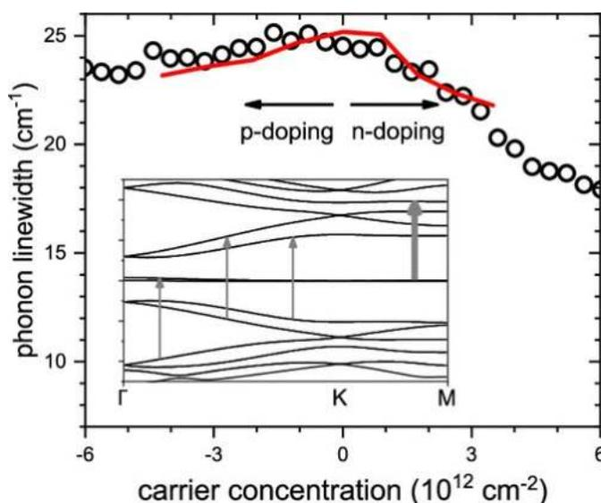
**Figure 1:** Gate-dependent G-band Full-Width-Half-Maximum in the magic-angle TBLG
