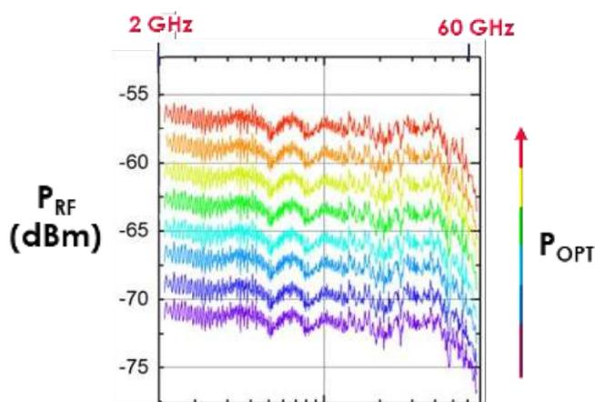
**Figure 2:** High frequency 1.55 $\mu$ m photodetection with a 7.5nm-thick PtSe<sub>2</sub> channel inserted in a coplanar waveguide. A 60GHz bandwidth photodetector is demonstrated.
