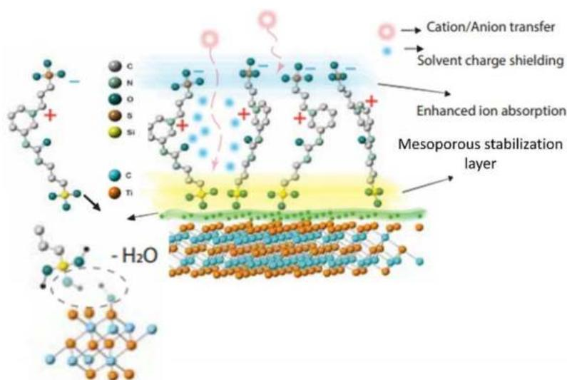
**Figure 1:** Schematic functionalization of MXene with Zwitterionic molecules.
