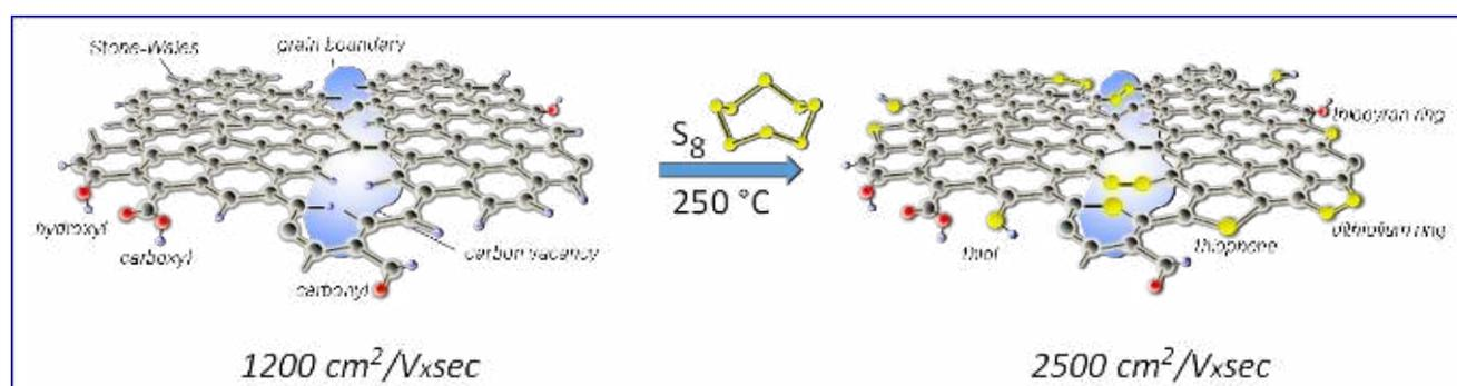
**Figure 1:** Schematic representation of CVD graphene as prepared and after thermal sulfurization process. The yellow spheres represent sulfur atoms. The different C–S bonding configurations inserted into the graphene network are evidenced as well as the typical carbon vacancies, grain boundaries and the Stone–Wales defects.
