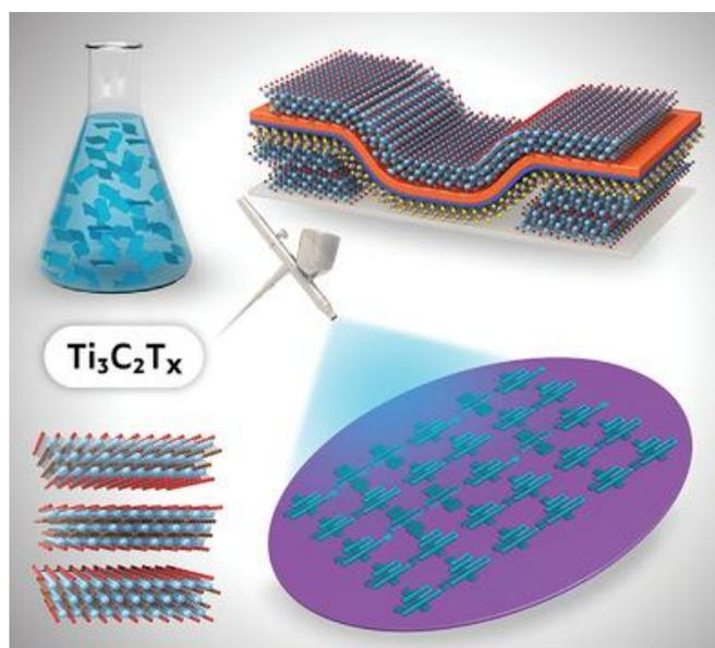
Figure 1:  $Ti_3C_2T_x$  MXene in wafer-scale integrated 2D electronics
