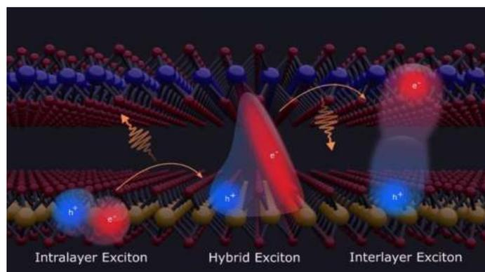
**Figure 1:** Sketch of the charge transfer process. Starting from an exciton localized in the bottom layer, phonon-mediated scattering to an hybrid exciton state (where e.g. the electron lives in both layers) allows for the transfer of the charge (here electron) to the upper layer resulting in a spatially separated interlayer exciton state.
