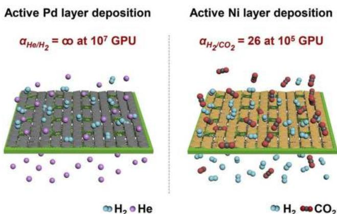
**Figure 1:** Schematic representation of Pd-coated for  $\text{He}/\text{H}_2$  (left) and Ni-coated membrane for  $\text{H}_2/\text{CO}_2$  (right) separation.
