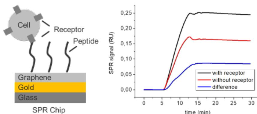
**Figure 1:** Binding of cells on biosensors with graphene and peptide coating. Left: Schematic sensor setup. Right: SPR signal as a function of time. Here, the binding of cells with and without receptors was compared. The difference between the two measurement curves gives the proportion of specific binding to peptides. The cell concentration was 275,000/ml in both cases.
