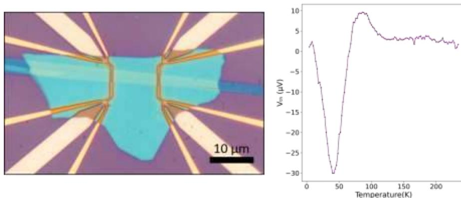
**Figure 1:** Left: Optical micrograph of a thermoelectric device. A few-layer CrSBr flake is stamped onto gold contacts and encapsulated by a thin hBN flake. Right: Thermovoltage as a function of temperature measured at zero magnetic field.
