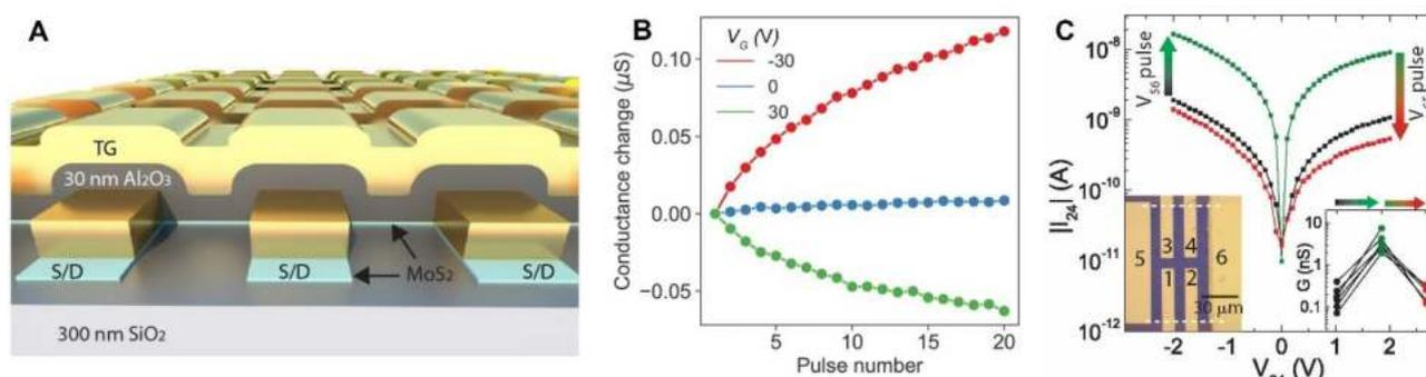
**Figure 1:** (A) Schematic of a dual-gated 2D memtransistor crossbar array. Adapted from Ref. 7. (B) The unipolar synaptic response of 2D memtransistors can be tuned from potentiation to depression as a function of the gate bias. Adapted from Ref. 8. (C) Multi-terminal 2D memtransistors show heterosynaptic responses between orthogonal contacts. Adapted from Ref. 5.
