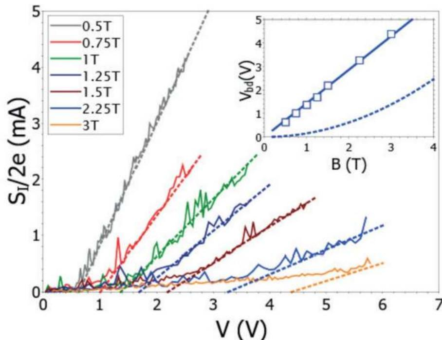
**Figure 1:** Breakdown shot noise as function of bias voltage, measured at a fixed charge carrier density  $n=2.10^{12} \text{ cm}^{-2}$  for magnetic fields between 0.5T and 3T in a graphene transistor. Breakdown is signalled by a strong increase of noise. Inset shows the linear increase of breakdown voltage with B-field (blue line corresponding to a constant breakdown velocity  $v_{BD}=0.14v_F$ ), that strongly deviates from the Zener inter-Landau-level tunnelling (dashed line).
