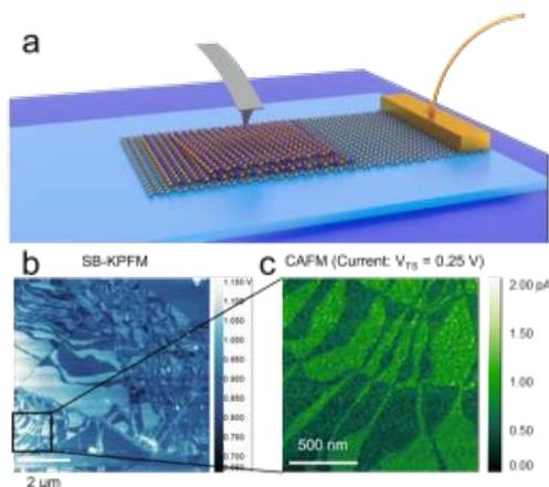
**Figure 1:** Parallel stacked hBN may be formed by breaking and restacking exfoliated layers mechanically (a). Once formed, these structures may be characterised using KPFM to map the morphology of ferroelectric domains (b). For sufficiently thin layers ( $\sim 0.6$  nm), tunnelling current may be mapped using CAFM.
