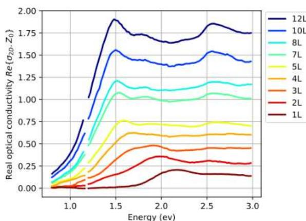
**Figure 1:** Optical spectroscopy of monolayer to quasi-bulk 12-layers exfoliated PtSe<sub>2</sub>. The high-energy plateau of the 2D real sheet conductivity  $\text{Re}\{\sigma_{2D}, Z_0\}$  (with  $Z_0$  the impedance of vacuum) scales with the number of layers. While 2D confinement explains the redshift of the peaks position with the thickness, a non-trivial and intrinsic mechanism is responsible for the slowly decaying low-energy absorption tail.
