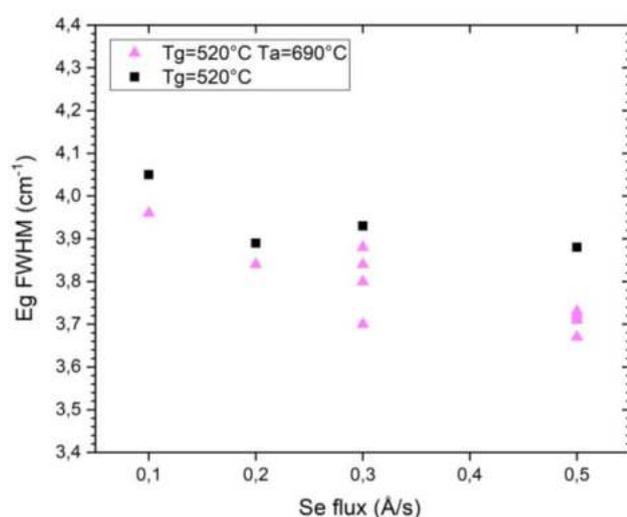
**Figure 1:** FWHM of Eg RAMAN peak of PtSe<sub>2</sub> films grown at T<sub>g</sub>=520°C with a post-growth annealing at T<sub>a</sub>=690°C (purple triangles) or without anneal step (black squares), under different Se fluxes.
