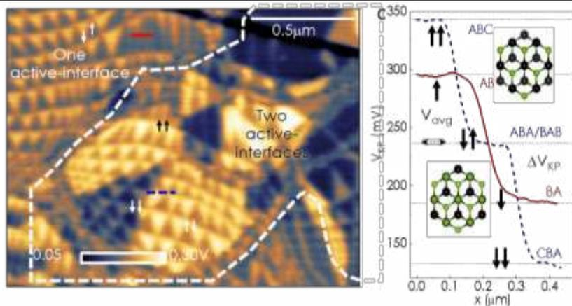
**Figure 1:** Electric surface potential of interfacial polarization in parallel TMD trilayers
