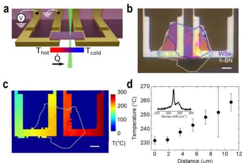
**Figure 1:** a) b) Schematic sketch (a) and optical image (b) of the device structure with a suspended hBN between two silicon heaters. c) Temperature map of Si when 6 V are applied on the right electrode. d) Gradient of temperature of WSe<sub>2</sub> along a line from the cold electrode to the hot one (inset: Raman spectrum of WSe<sub>2</sub>) All scales bar : 10 microns
