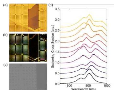
**Figure 1:** NiPS<sub>3</sub> magnetic nanoantenna on gold. (a) Bright field and (b) dark field optical images. (c) SEM image. (d) Dark-field scattering spectra.
