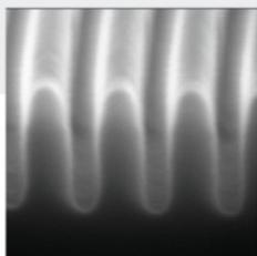
25 nm wide Si trenches etched to 110 nm depth by ALE.
