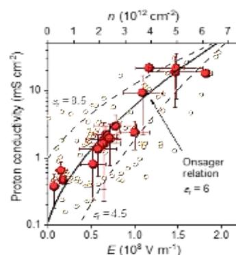
**Figure 1:** Proton conductivity through graphene electrode where  $n$  is the carrier density. Bottom x-axis, is Electric field strength on graphene electrode. Solid curve, best fit of Onsager model to data. Dotted curves, Onsager model for different dielectric constant.
