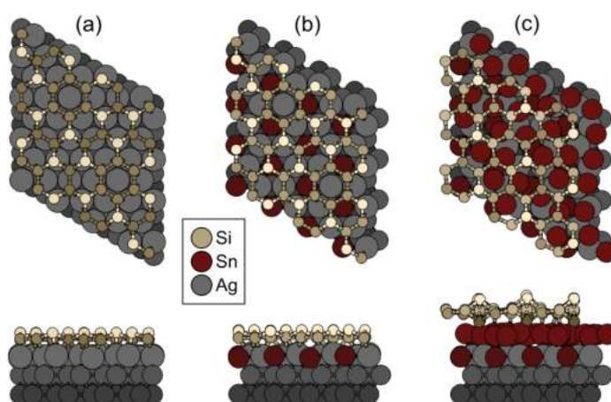
**Figure 1:** Structural models of silicene grown on (a) Ag(111), (b) SnAg<sub>2</sub>/Ag(111), and (c) stanene/SnAg<sub>2</sub>/Ag(111).
