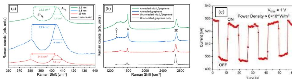
**Figure 2:** a) Raman spectra of MoS<sub>2</sub> with the separation between the A<sub>1g</sub> and E<sub>12g</sub> peaks reducing with deposition thickness. (b) Raman spectra of graphene showing the 2D peaks remain after annealing. (c) photo-illumination cycles showing induced photocurrent with a switching laser source
