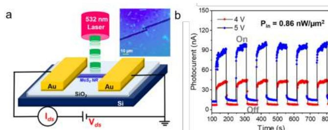
**Figure 2:** (a) Schematic of the MoS<sub>2</sub> nanoribbon device under 532 nm laser illumination and (b) ON/OFF photo response of the nanoribbon.
