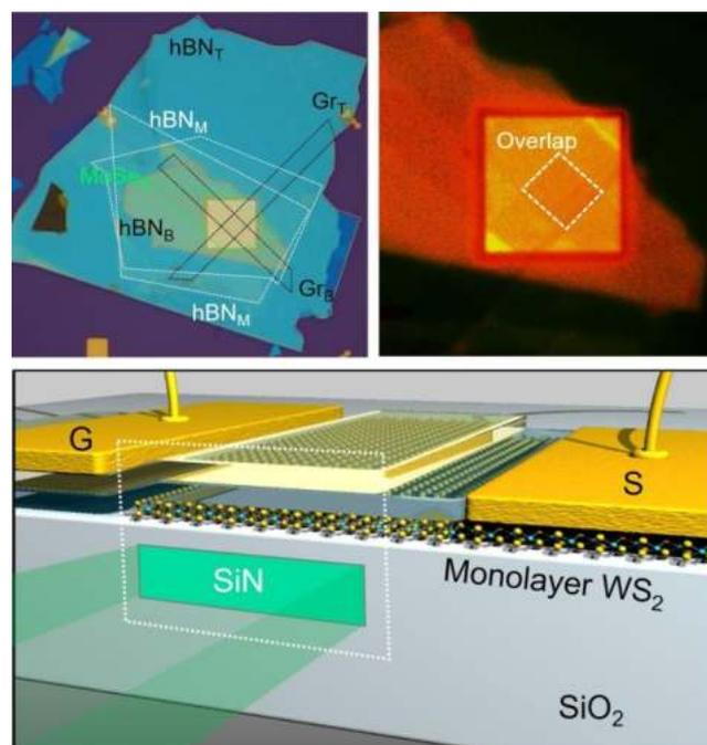
**Figure 1:** 2D materials-based optoelectronic devices and those integration into Si photonics platform. Light emitting device using MoSe<sub>2</sub> (top) and WS<sub>2</sub>-SiN hybrid photonics for low-loss modulation (bottom).
