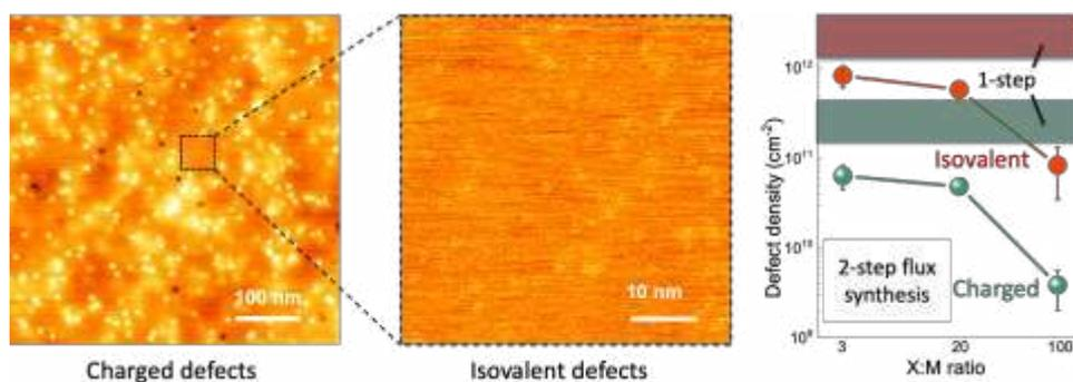
**Figure 1:** Defects in flux-grown TMDs. Left, large-scale STM image showing charged donor (bright) and acceptor (dark) defects. Middle, smaller-scale STM image showing isovalent defects. Right, density of both defect types as a function of selenium:tungsten ratio.
