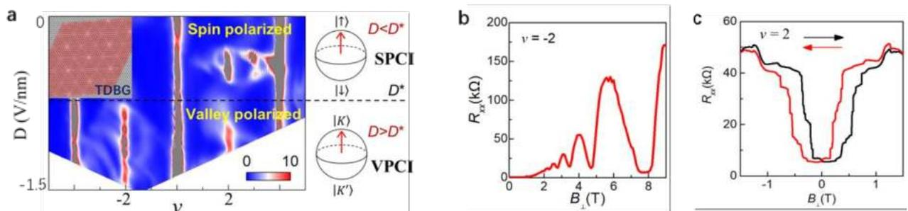
**Figure 1:** (a) A colour mapping of resistance as a function of moiré band filling ( $\nu$ ) and displacement field ( $D$ ) in TDBG, and SPCI and VPCI denote spin polarized and valley polarized correlated insulator, respectively. (b) Unconventional quantum oscillations in the VPCI at  $\nu = -2$  ( $D > D^*$ ). (c) Evidences of the first-order phase transitions and ferromagnetism in the SPCI at  $\nu = 2$  ( $D < D^*$ ).
