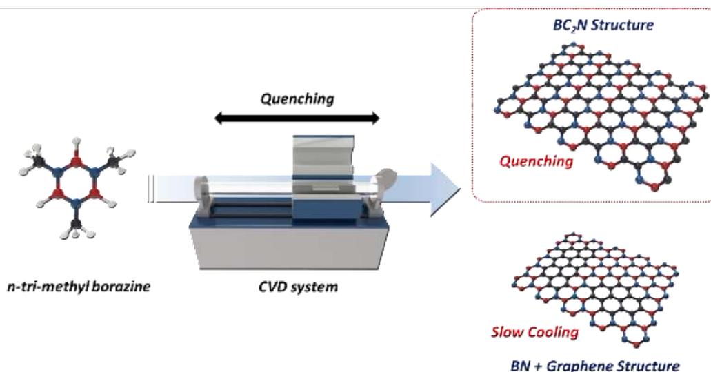
**Figure 1:** Schematic diagram of  $h$ -BC<sub>2</sub>N synthesis.
