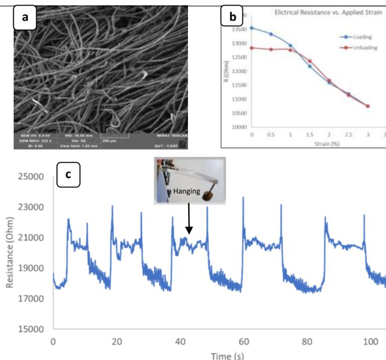
**Figure 1:** (a) SEM image of the graphene coated nonwoven fabric, (b) Electrical Resistance vs. Applied Strain (c) the static response of the strain sensor under strain
