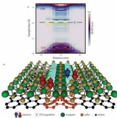
**Figure 1:** Band gap renormalization over a 1D defect within WS<sub>2</sub> realized at the atomic scale.
