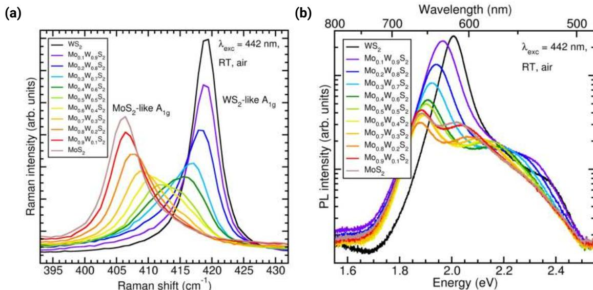
Figure 1: Raman spectra (a) and PL spectra (b) of Mo <sub>$x$</sub> W <sub>$1-x$</sub> S<sub>2</sub> monolayers with different concentrations.
