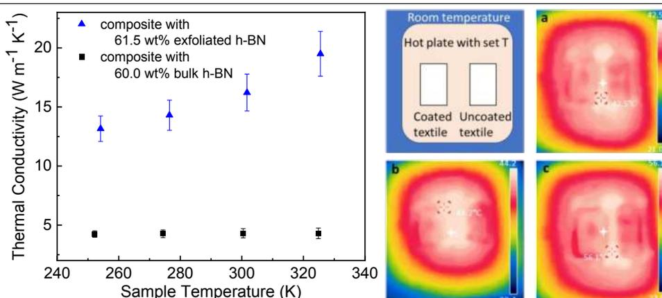
**Figure 1:** Left: Thermal conductivity of the exfoliated and bulk h-BN assisted composites; Right: Comparative temperature measurements between the coated textile and the uncoated textile.
