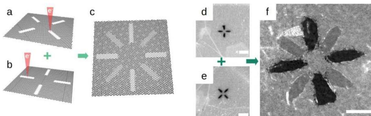
**Figure 1:** (a-c) Schematic of cutting a pattern into individual graphene layers (a,b) followed by aligned stacking (c). (d-f) Experimental realization, (d,e) SEM images of crosshair structures cut into graphene, (f) Dark-field TEM image showing the assembled structure, set for highlighting one of the two layers. Scale bars are (d,e) 500 nm and (f) 200 nm. Adapted from Ref. 1.
