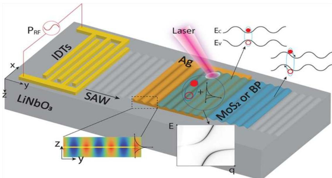
**Figure 1:** Schematic of the proposed plexciton launcher where a SAW generated by interdigitated transducers (IDTs) placed on top of a piezoelectric substrate leads to the coupling between metal plasmons and excitons in 2D semiconductors by means of the dynamic surface rippling and bandgap modulation.
