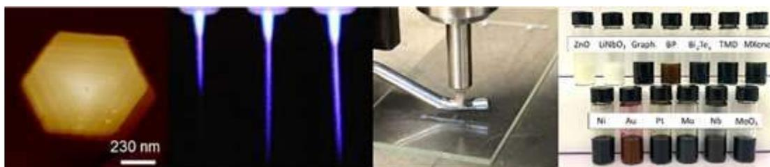
**Figure 1:** Examples of inks and printers for direct writing of electronics. Left to right shows thermoelectric flakes, plasma jet printing, aerosol jet printing, and library of developed inks.
