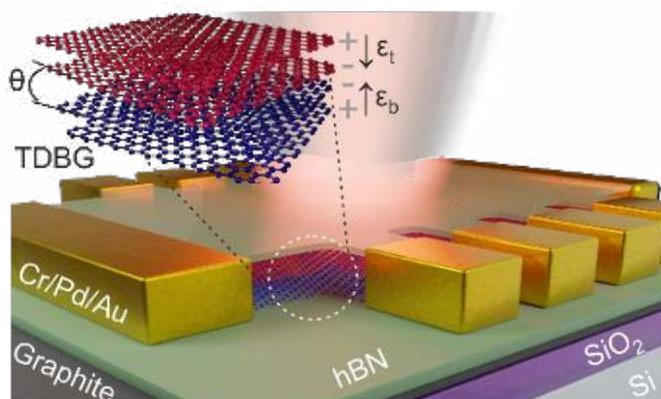
**Figure 1:** Schematic of photocurrent experiments in twisted graphene heterostructures
