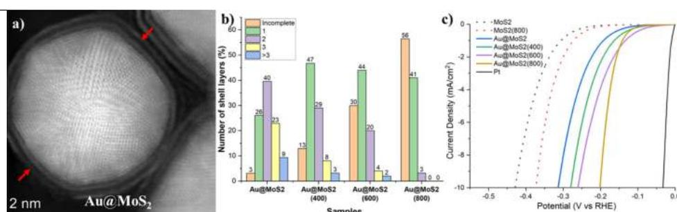
**Figure 1:** Aberration-corrected STEM image of the initial Au@MoS<sub>2</sub> sample, b) Evolution of the number of shell layers c) LSV curves obtained in 0.5 M H<sub>2</sub>SO<sub>4</sub> at 10 mV·s<sup>-1</sup>.
