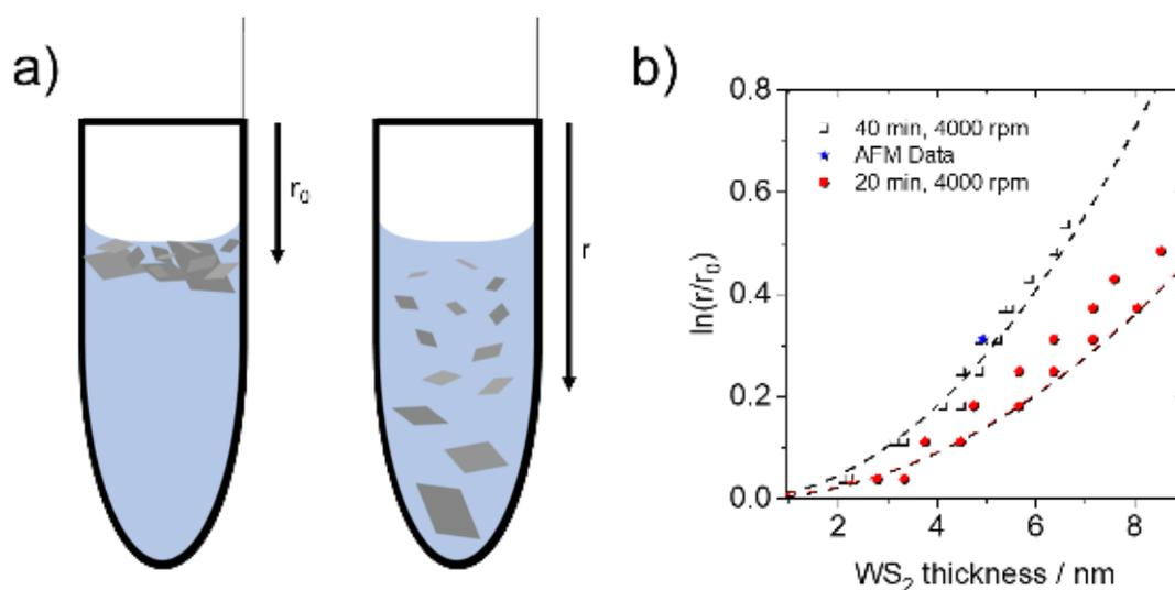
**Figure 1:** a) Schematic of band sedimentation process to separate nanoflakes according to size. b) Measured distribution of tungsten disulphide flake sizes down centrifuge tube matching the theoretically predicted distribution (dashed lines).
