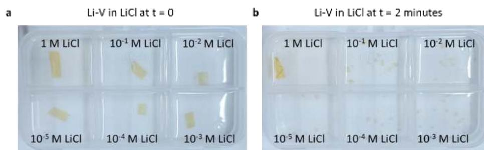
**Figure 1:** The stability of Li-Vermiculite membrane in aqueous LiCl solution. Li-V membrane in various concentrations of LiCl ranging from 1 M to  $10^{-5}$  M at time (a)  $t = 0$ , and (b)  $t = 2$  minutes.
