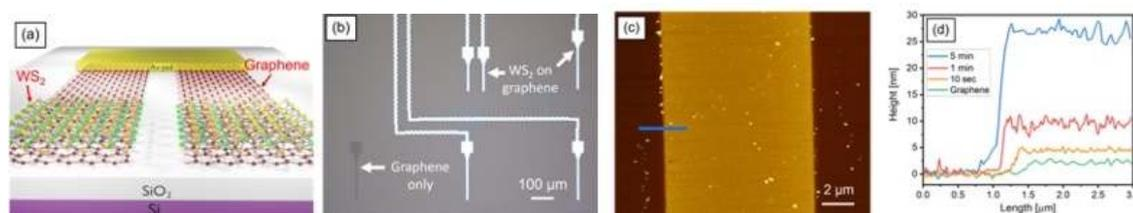
**Figure 1:** (a) A schematic illustration of WS<sub>2</sub> deposited on patterned graphene that is biased through Au contact pad. (b) An optical microscope image. (c) AFM topography images of WS<sub>2</sub> deposits on graphene for 1 minutes. (d) Line profiles showing total step height.
