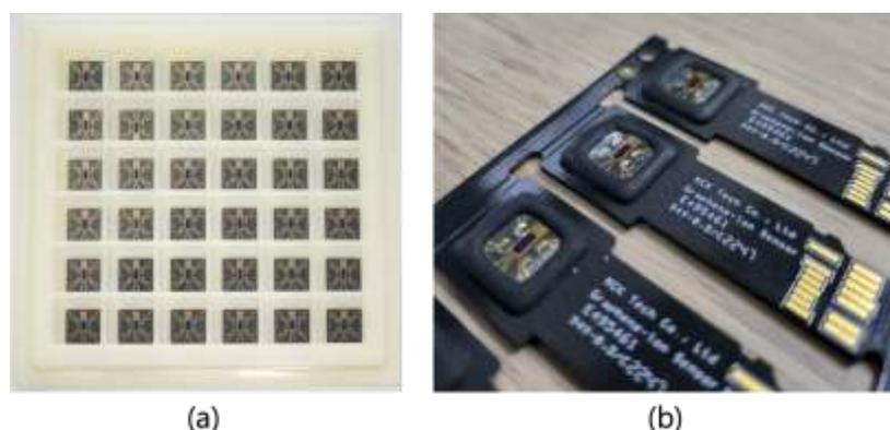
**Figure 1:** (a) Graphene FET (G-FET) (b) Packaged G-FET
