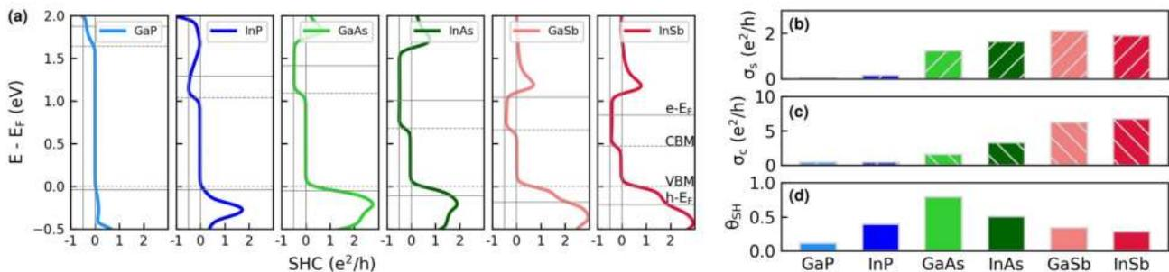
**Figure 2:** (a) Spin Hall conductivities of 6 III-V monolayers. The dashed lines denote the conduction band minimum and valence band maximum of intrinsic semiconductors, and the solid lines indicate the position of Fermi energy after electron doping and hole doping, respectively. (b)-(d) The spin Hall conductivity, charge conductivity, and spin-charge-conversion efficiency after hole doping of 2 × 10<sup>13</sup> cm<sup>-2</sup>.
