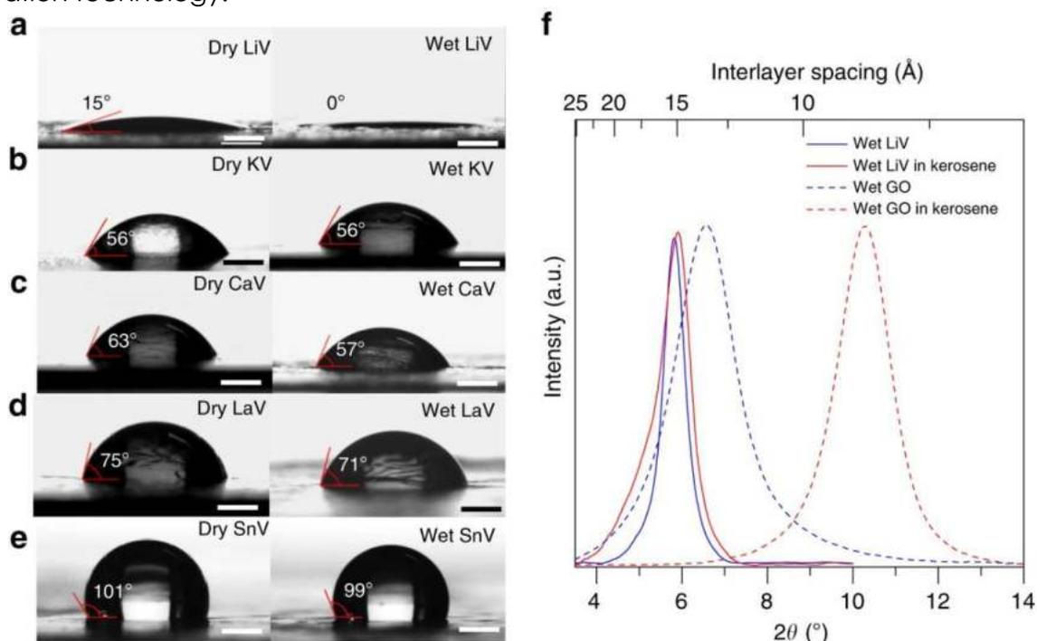
**Figure 1:** Wetting properties of vermiculite laminates: (a–e) Water contact angle of lithium vermiculite (LiV), potassium vermiculite (KV), calcium vermiculite (CaV), lanthanum vermiculite (LaV), and tin vermiculite (SnV) -laminates in dry and wet states. Scale bar, 750  $\mu\text{m}$  f) XRD from wet LiV laminate before and after immersing in kerosene for a week along with XRD spectra of a reference GO membrane tested at identical condition.
