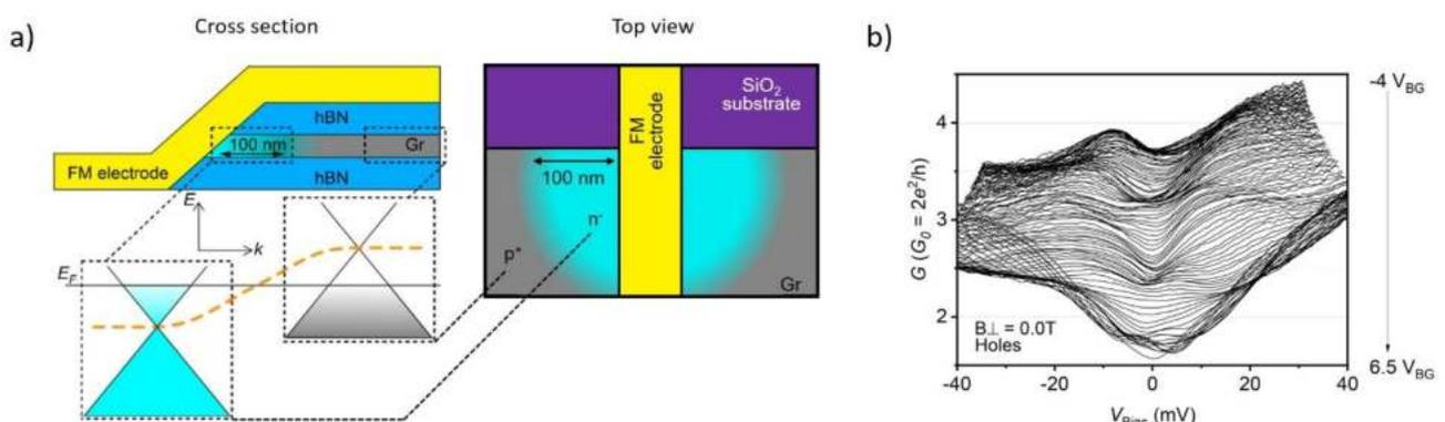
**Figure 1:** (a) 2D cross section and top view of the 1D contact architecture. Figure adapted from [1]. (b) Bias spectroscopy conductance measurement of a 1D contact, for hole transport ( $V_{BG} > V_D$ ) without an applied magnetic field
