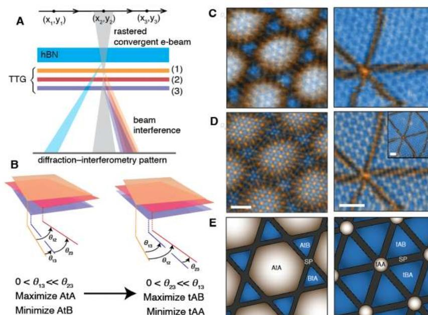
**Figure 1:** (A) Schematic of the 4D Scanning Transmission Electron Microscopy (STEM) approach, wherein beam interference is used to extract stacking order. (B) Schematics of layer alignment in TTG. (C) Maps of local atomic stacking from the larger moiré pattern only. (D) Local atomic stacking obtained from considering all three graphene layers. (E) Qualitative schematic illustrating the atomic reconstruction observed.
