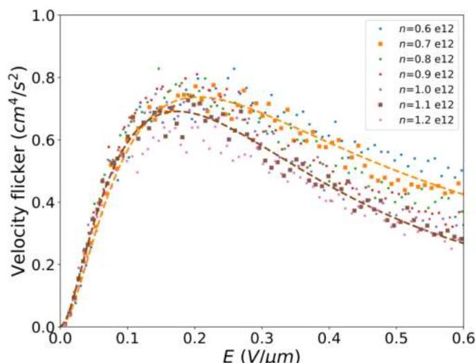
**Figure:** Velocity flicker noise measured in a high-mobility graphene transistor, as function of bias electric field for different dopings, demonstrating a quasi-scaling. The noise level presents a bell-shape with respect to bias, that is accounted for by a modified Hooge formula (dashed lines) in the non-linear velocity saturation regime.
