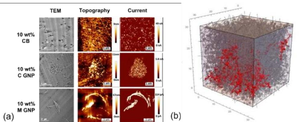
**Figure 1:** a) TEM image as well as topography and current mapping obtained from conductive-AFM of composites and (b) example Monte-Carlo simulation of hybrid system with the percolated pathway highlighted in red.
