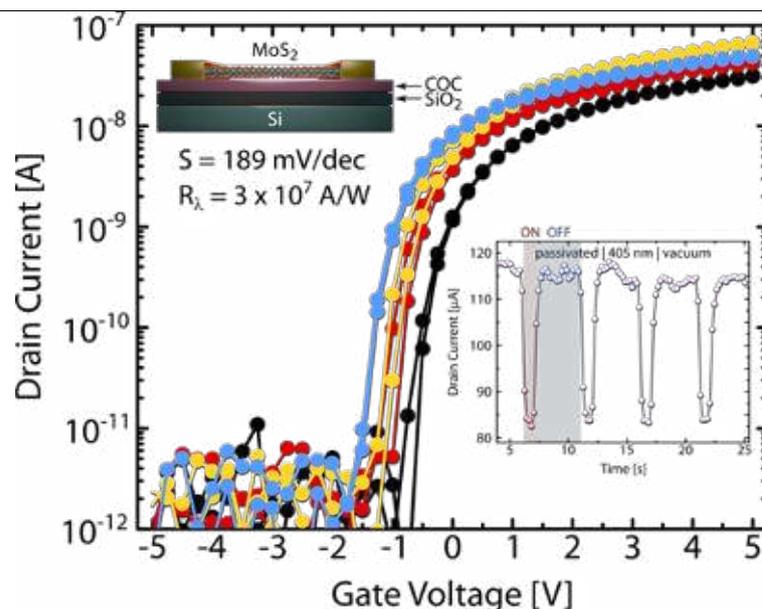
**Figure 1:** Performance of monolayer MoS<sub>2</sub> based electronic and optoelectronic devices on SiO<sub>2</sub> gate dielectric passivated with cyclic olefin copolymer.
