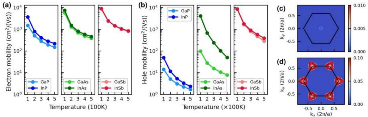
**Figure 1:** (a)-(b) Temperature-dependent electron and hole mobilities of 6 III-V monolayers. (c)-(d)  $k$ -resolved scattering rate of InSb electron transport and GaP hole transport, respectively.
