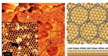
**Figure 1:** 2D sp-sp<sup>2</sup> carbon network on Au(111). STM and theory model
