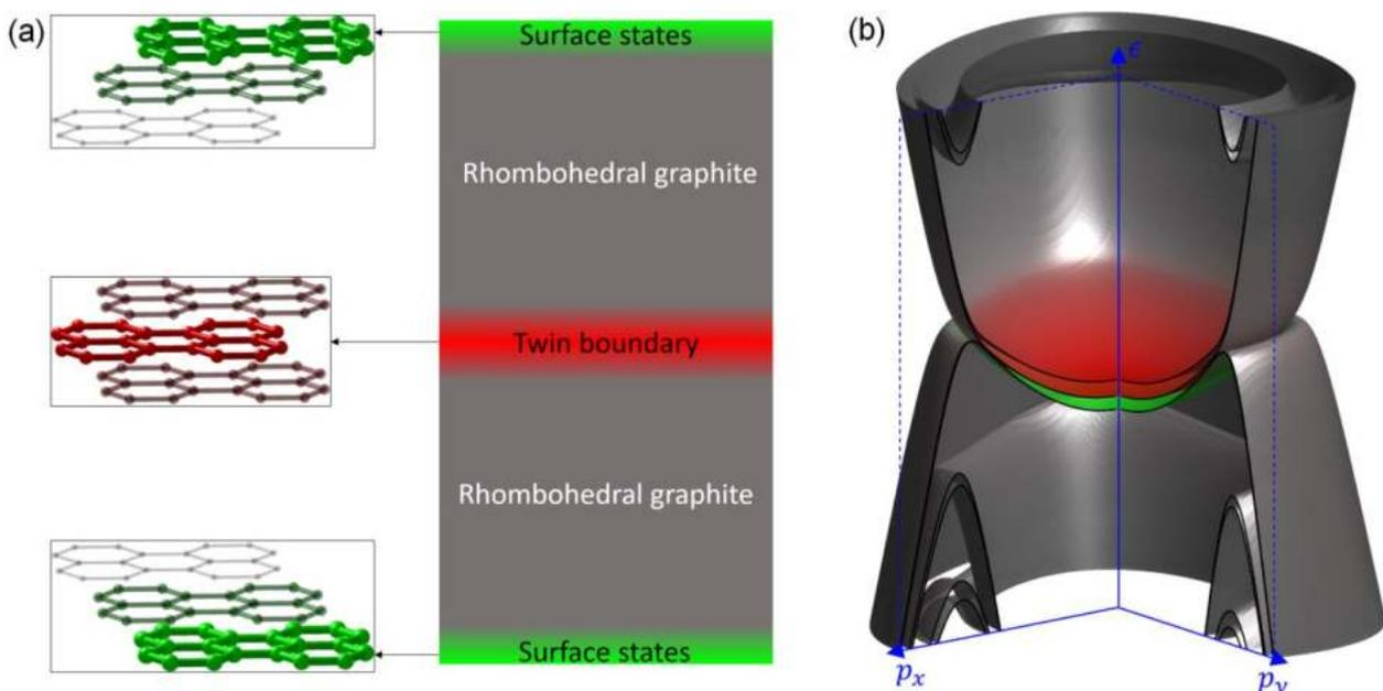
**Figure 1:** (a) Rhombohedral graphite with a twin boundary. The top and bottom insets present the characteristic ABC-stacking of rhombohedral graphite, while the middle inset presents the only ABA-stacking order in the film. (b) Band structure of rhombohedral graphite with a twin boundary, coloured according to the localisation of the wavefunction. The red bands, localised inside the film, could induce correlated phases protected from environment.
