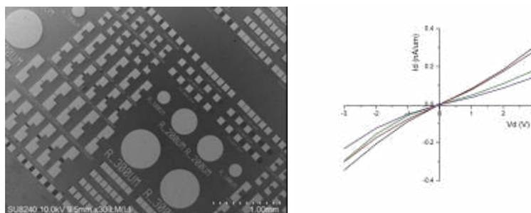
**Figure 1:** 5nm CVD MoTe<sub>2</sub> -FET SEM image and electrical measurement result
