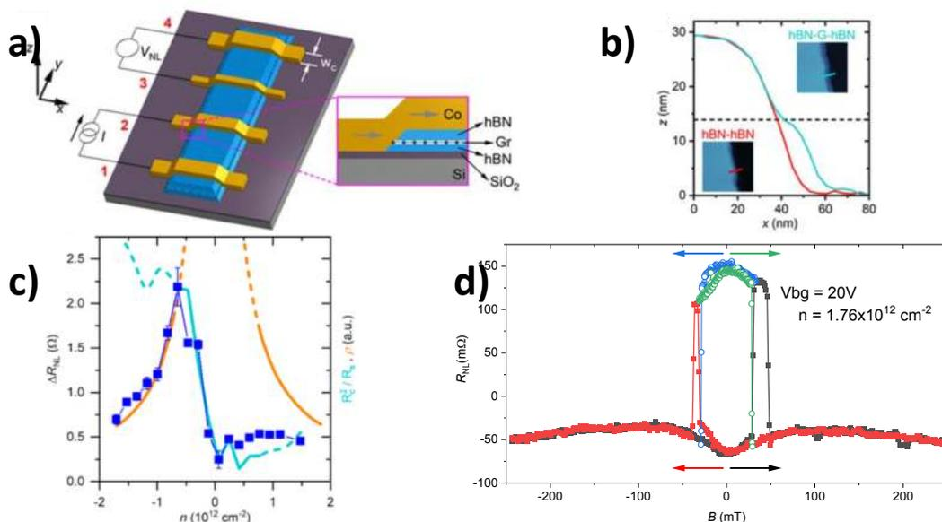
the 1D contact. (b) AFM profile of the edges of a device comparing hBN-only vs hBN-encapsulated graphene. (c) Spin signal  $\Delta R_{NL}$  as a function of charge carrier density, compared to trends in resistivity (orange) and the contact-to-spin-resistance ratio (cyan). (d) Spin-valve measurement showing a Hanle-like baseline revealing presence of spin components in-plane and out-of-plane.
