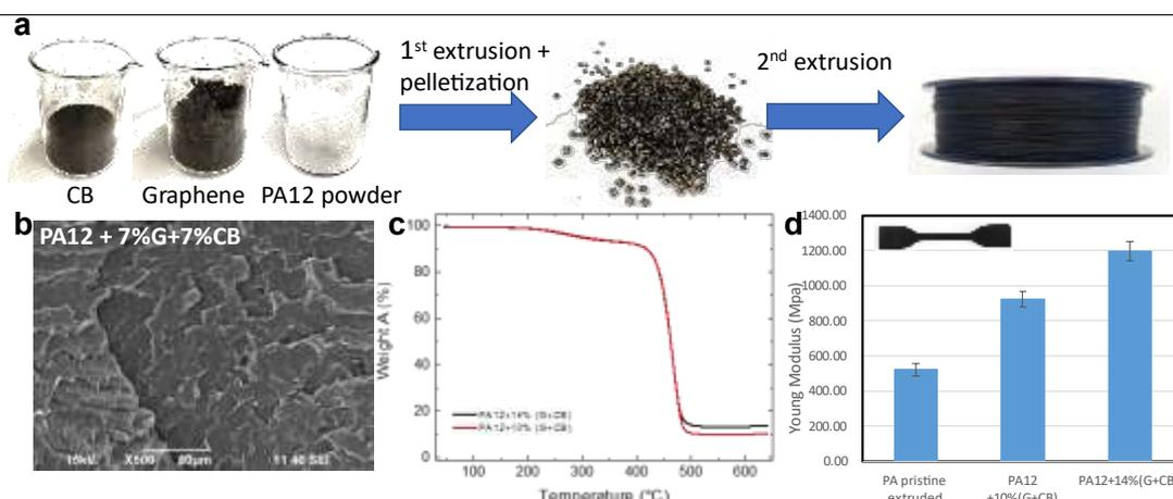
**Figure 1:** (a) Scheme of the GPCs filament production. (b) Scanning electron microscopy image of PA12+14% (FLG+CB). (c) thermogravimetric analysis of PA12+10% and 14% (FLG+CB) (d) flexural modulus of pristine PA12 and of the composite PA12+10% and 14% (FLG+CB).
