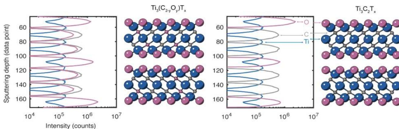
**Figure 1:** SIMS depth profiles of multilayer  $\text{Ti}_3\text{C}_2\text{T}_x$  MXene samples. Samples produced with conventional processes (left) show significant levels of oxygen in the carbon layer, qualifying them as oxycarbides. Pure carbides can be obtained with modified production procedures (right).
