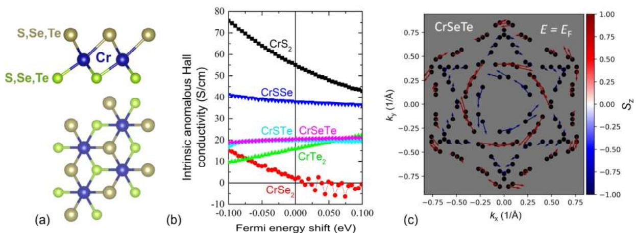
**Figure 1:** *Ab initio* calculations of CrXY [ $X, Y \in \{S, Se, Te\}$ ] monolayers in the 1T phase. (a) Crystal structure of the monolayer 1T phase. (b) Calculated intrinsic anomalous Hall conductivity as a function of Fermi energy shift for the 6 materials. (c) Spin texture at the Fermi surface of a monolayer CrSeTe as a function of the in-plane wave vectors. The asymmetrical structure leads to an effective out-of-plane electric field and resulting Rashba-like spin-momentum locking.
