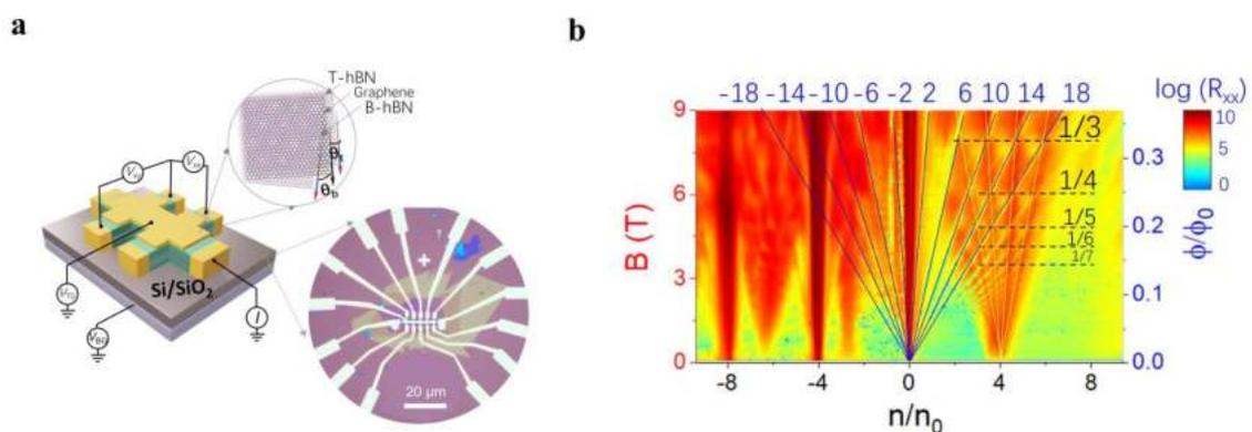
**Figure 1: Double-aligned hBN/graphene/hBN heterostructure.** **a**, Schematics of the dual-gate device with supermoiré lattice. **b**, Landau fan diagram showing the Brown-Zak (BZ) oscillations in a perfect double-aligned device.
